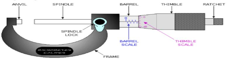
An object to be measured is placed between the anvil and the spindle. The thimble is adjusted until the object is almost gripped between the anvil and spindle. Turning the ratchet then adjusts the grip of the micrometre to the same tightness each time.
